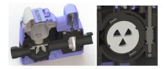
The valve is implemented with a set of sliding rotary plates actuated by a precision micro-motor and gearhead. These plates are constructed with a Teflon composite with very high tolerances. The design and materials of the valve ensure low friction/low power operations for long term performance. One of the plates rotates to adjust the aperture of the valve as shown in the diagram above.
